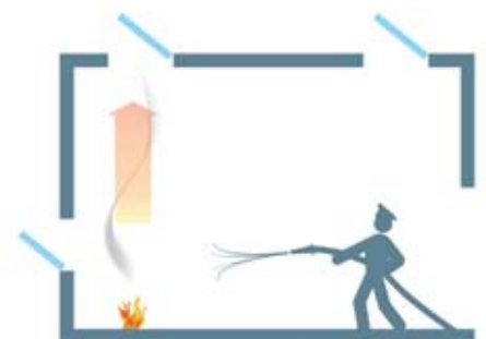
3. The smoke-free layer allows safe access for the fire to be fought and extinguished.
